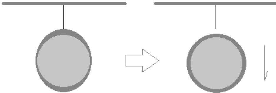
Suspended steel ball before and after the wire is cut
